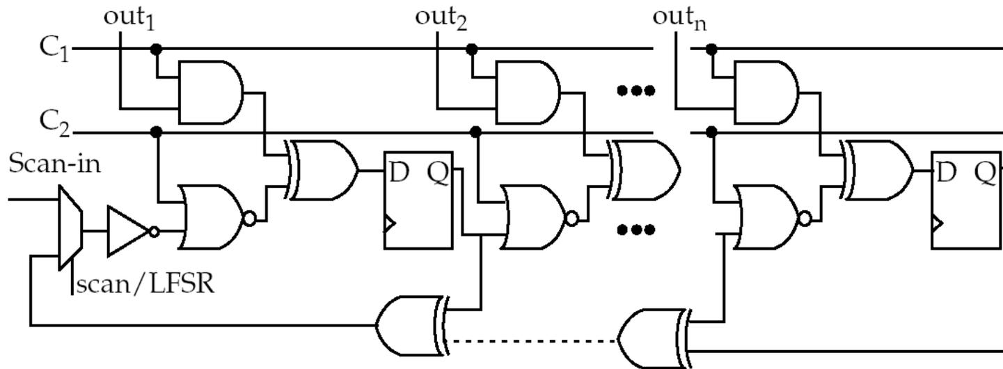
C<sub>1</sub> and C<sub>2</sub> configure as a **shift register** for scan (00), an **LFSR** (00), **MISR** (10) a **Normal** (11).
