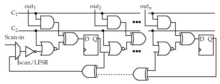
C<sub>1</sub> and C<sub>2</sub> configure as a **shift register** for scan (00), an **LFSR** (00), **MISR** (10) a **Normal** (11).
