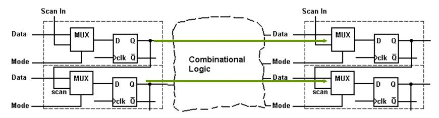
Step 2 : Operate for one clock cycle
